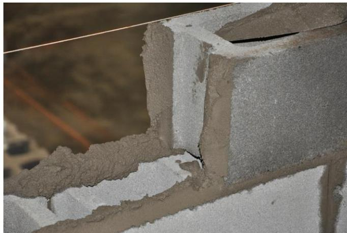
Figure 3A – “Hollow” CMU unit laid in a full bed joint with a full head (end) joint
